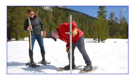
Other field work undertaken during the summer includes installing, operating, and evaluating experimental equipment to provide cooperating agencies with information for designing future automatic snow data collection networks.
