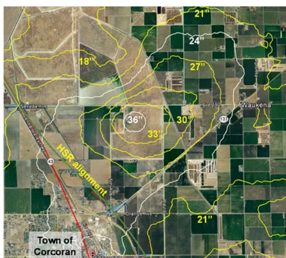
Figure 4-1: Local subsidence bowl developed using data acquired from June 2007 to December 2010 with a maximum subsidence of 36 inches, and 18 to 21 inches around its periphery, in the vicinity of the HSR Alignment. InSAR data from Farr et al., 2015.
