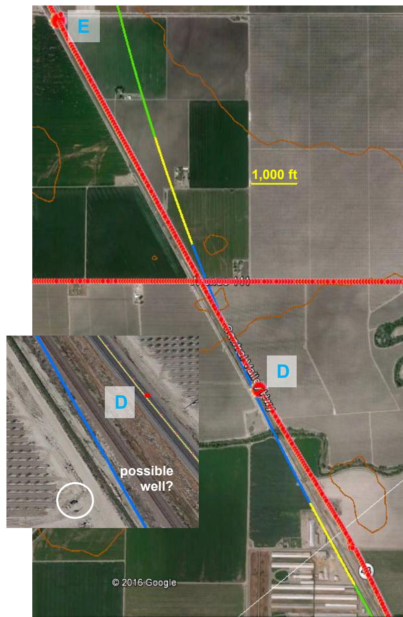
Tule River Viaduct Area Approximate location of anomalous elevation change consistent with historic (but not current) well pumping at point 'D.' There is a possible indication of a well being present in the vicinity of point 'D.' However, point 'D' is not the nearest RTK point to the feature.
