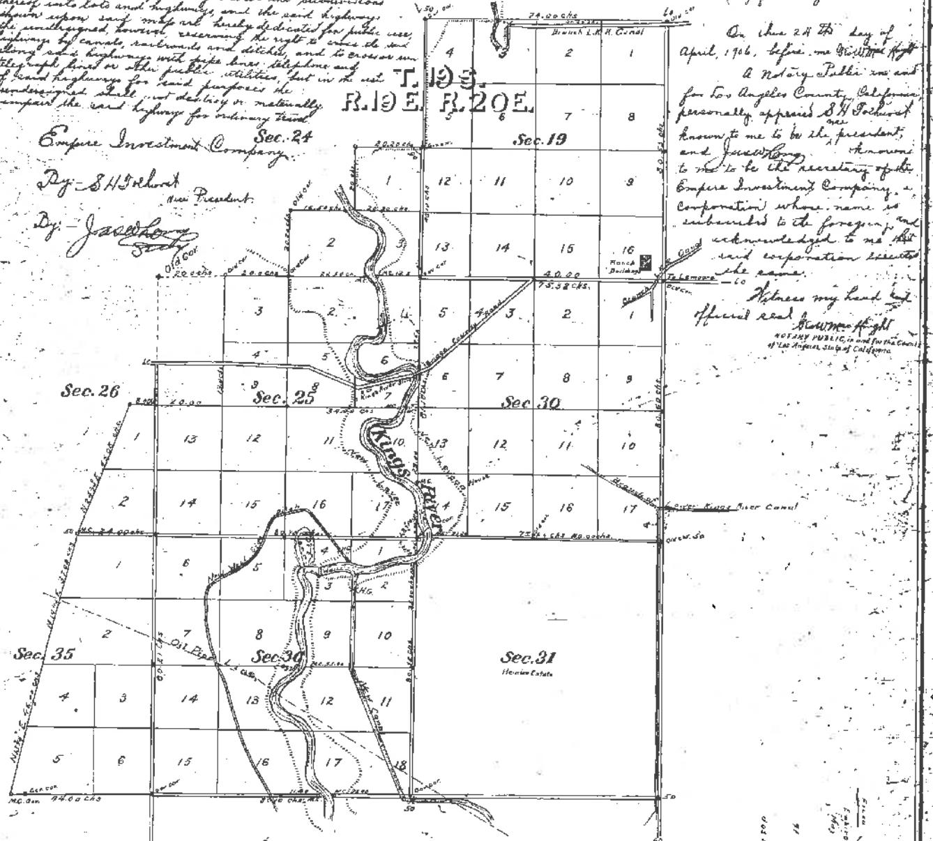
Sec. 1/4 Sect. & Meander Cor's Are Marked in The Field With 2 inch Iron Pipes
